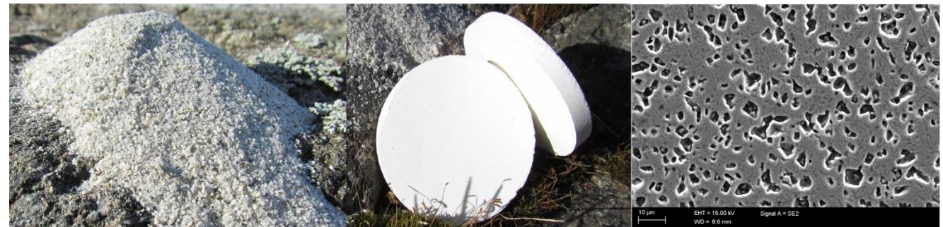
Successfully synthesized white mullite based ceramic pieces utilizing Mo ore tailings as raw material source.
