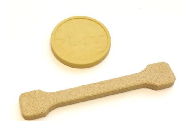
Powder injection moulded and sintered parts made of a mine tailings.
